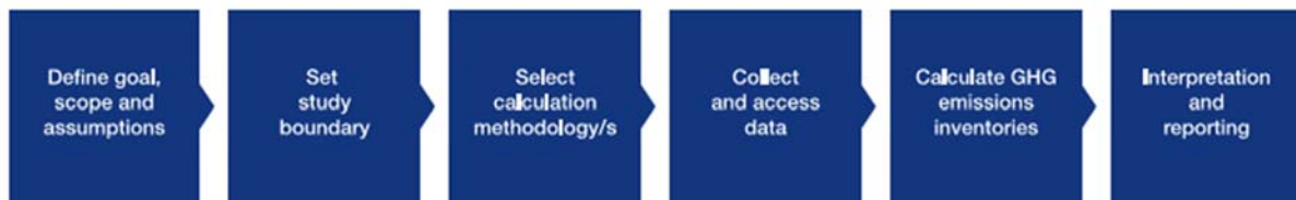
Figure 7.4 Principal steps of carbon emissions quantification (from PAS2080)
